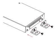
Install the brackets onto the position as desired using the screws (not included).
